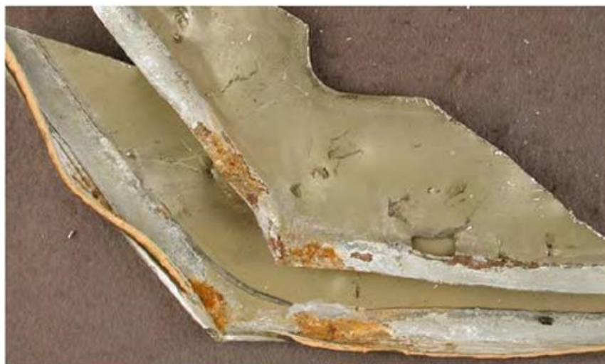
Figure 4. Superficial corrosion – 10-50 % of the hem flange of a hood covered with rust.
