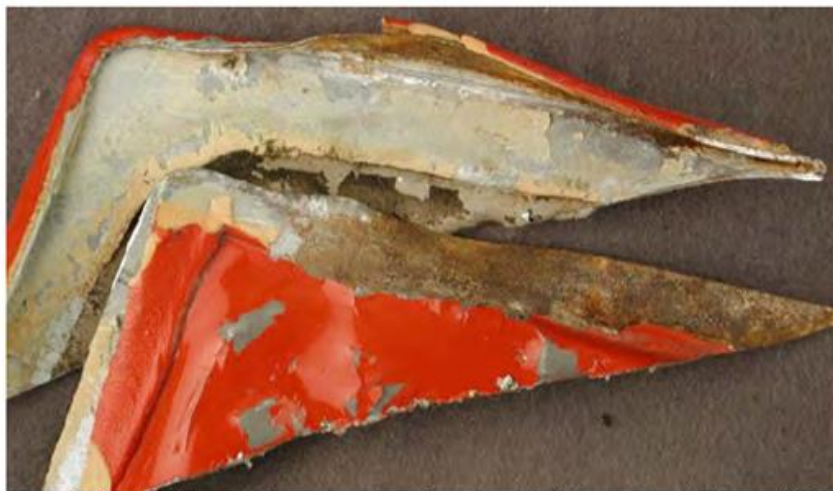
Figure 6. Considerable corrosion – corrosion with no deep pits but corrosion attack on > 50\% of the hem flange of a door
