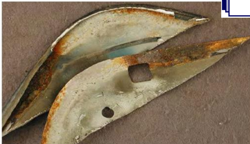
Figure 5. Considerable corrosion – corrosion with deep pits ( >150\ \mu\text{m} ) in the hem flange of a door.
