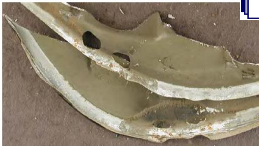
Figure 3. Insignificant corrosion – small rust spots on the hem flange of a door.
